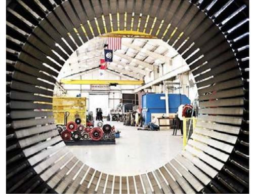
*Louis Allis can utilize a customer's existing motor frame and replace internal components, like this freshly manufactured core, ready to be wound.*
